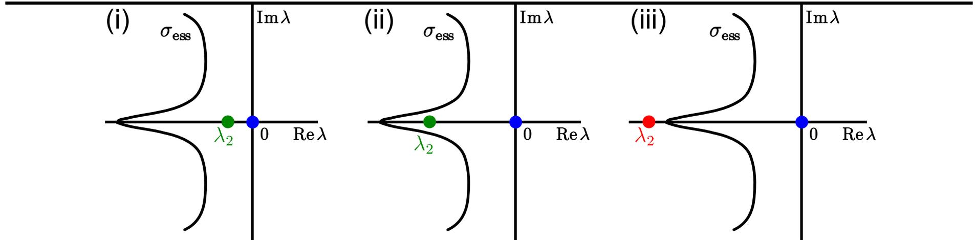
**Situation (i):**  $\lambda_2$  is an eigenvalue to the right of essential spectrum. Perturbations that change only the position of the back will decay without interacting with the front.
