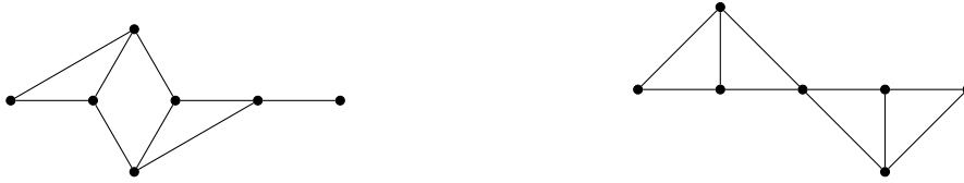
(a) Graph G_1 with \kappa_e(G_1) = 1 and \text{Rel}(G_1) = 1 - q + o(q) for q \rightarrow 0
