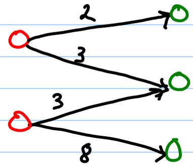
Bepaal  $u_i, v_j$  door te gebruiken dat  $u_1 = 0, \bar{c}_{11} = \bar{c}_{12} = \bar{c}_{22} = \bar{c}_{23} = 0$
